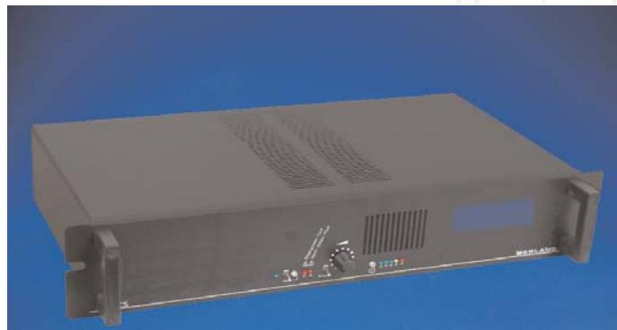
The CSD allows the surveillance of 8 Amplifiers and 8 speaker lines. The system needs the addition of an End of Line element EFLD.
